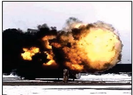
**Controlled demonstration showing the explosive potential of 52 lbs. (approx. 5-gallon pail) of PRB coal dust.**
